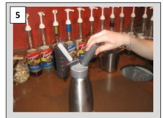
PLACE A SECOND CO2 CHARGE INTO CANISTER. LEAVE IN PLACE
